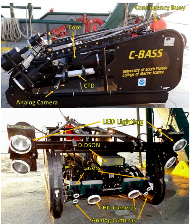
Above: Deploying the C-BASS off the deck of the R/V Weatherbird II (left) Images of the C-BASS (right).
